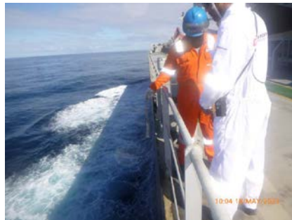
Sounding around the vessel using hand lead line
