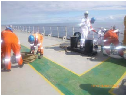
Rigging of Pilot Ladder
