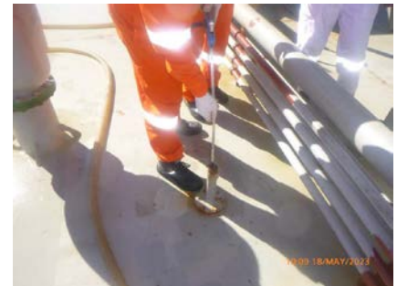
Sounding all ballast tanks
